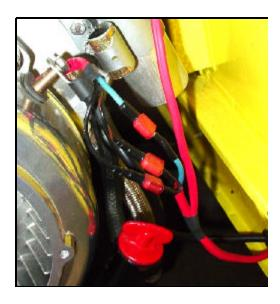
This gravure shows the small ignition harness that feeds the Dynastart and coil. Those quick connect spade lugs sit just above the dipstick. Two lugs were added to the coil wires as well.
