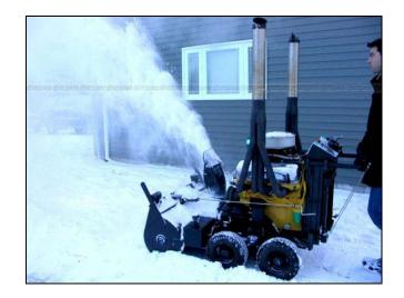
In order to get those two snowed-in Isettas at the top of Page One uncovered, we've enlisted the services of this **V-8 powered snow blower**. This bad boy is based on a **big-block 454 Chevy** motor cranking 412 HP. It'll throw snow 50 feet at 3,500 RPM's. Check out all the action at <u>www.v8snowblowers.com</u>. Also click on the "Gas Blender" link for a sneak preview of the **highperformance blender** they're whippin' up.
