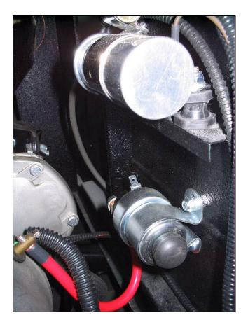
Richard Lewis has been keeping ALCN abreast of his rally Isetta resto. Regular readers already know he's spared no detail on this project. Here's a shot of the rubber-mounted coil and separate solenoid ala firewall. Given the fact that your editor had to re-install the coil on his Isetta twice due to engine vibration, this looks like a better idea all the time.
