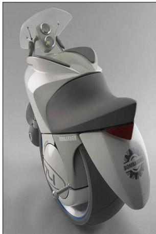
For our last entry, **Wayne Graefen** sent us this blurb on the **Embrio** one-wheeled motorcycle. This baby runs off of a hydrogen fuel cell system. At 12.5 mph, the front "landing gear" retracts and you're in unicycle mode. No mention of being able to juggle bowling pins as a requirement.
