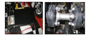
On the right, we've got some genuine BMW guibos (drive donuts for the rest of us) to beef up the drivetrain. Below right are the cool rally lights. On the left is a shot of a custom-machined tow/tiedown hook mounted on the chain drive. Neat!
