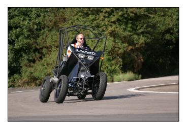
or without, this is one neato ride! **Scott Isensee** sent us the above pix and article on the **NARO** concept vehicle. It's designed for city use as a personal commuter, a taxi or a delivery vehicle, is intended to return over **100 miles per gallon** from a 400 cc, single-cylinder, 4-valve gasoline engine with a maximum of 20 HP.
