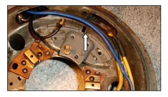
Here you can see the small oblong notch in the Dynastart housing just above the points bracket. The center V-notch sits just to the right of it at the bottom.
