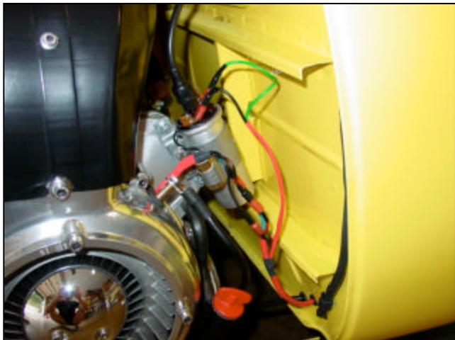
*Fresh ignition wiring harness with quick connect spade lugs. Note terminal that has been soldered onto starter cable. A 6mm bolt and lock washer secures the cable, ala BMW 600. This is done in lieu of placing cable through hole in side of post.*
