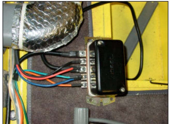
*New Nosso voltage regulator from Isetta John along with new ignition wiring harness. The VR is just slightly wider than the factory mounting brackets but can be fastened securely on one side. This also gives an extra margin of clearance between the terminals and that heater with plenty of clearance on right for the seat.*
